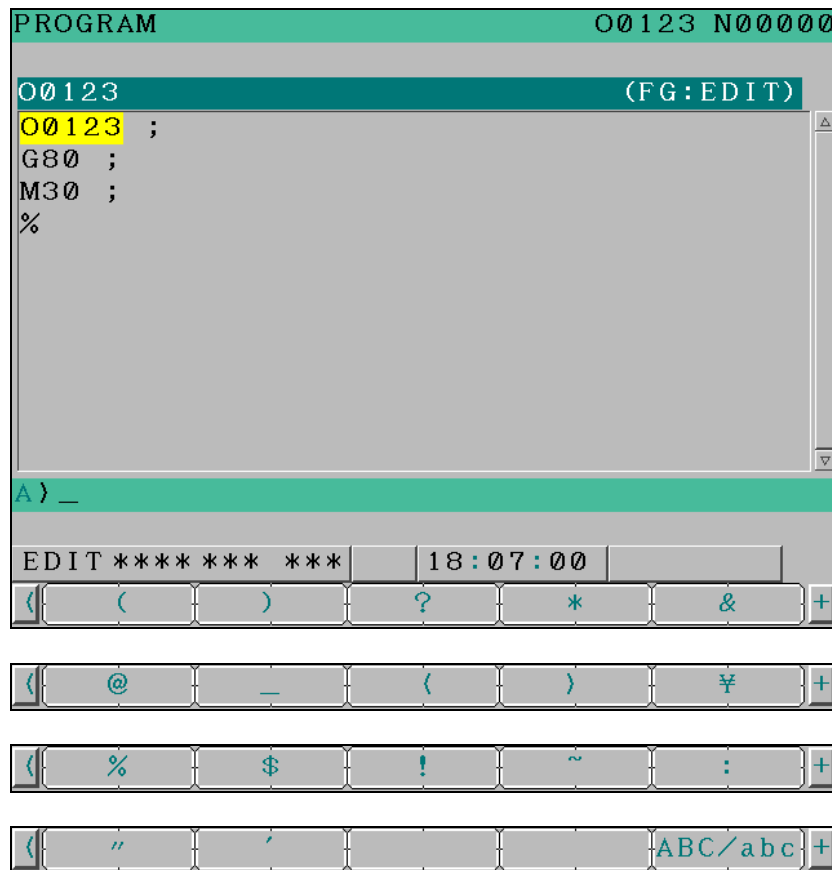
Fig. 10.11 (a) Compact-type MDI key input
